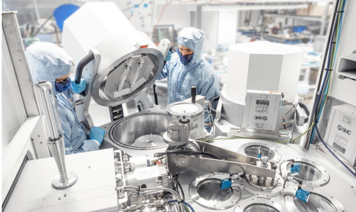
Fully automatic Flextura PVD Cluster system - designed and produced by Polyteknik AS
