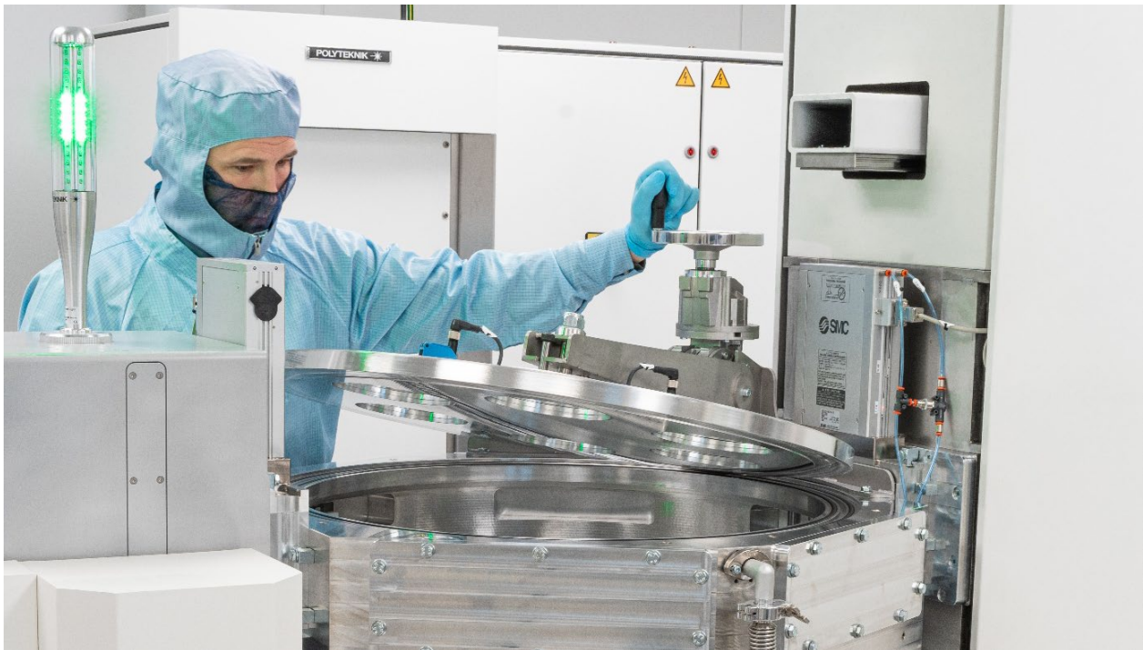
Fully automatic Flextura PVD Cluster system - designed and produced by Polytechnik AS
